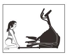
1. At the rear of the machine squat down and grasp the rear stabilizer bar.
